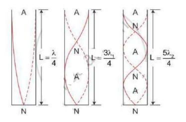
In the first mode of vibration of the air column, there is one node and one antinode as shown in the figure above.
