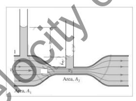
Let  $A_1$  and  $A_2$  be the cross-sectional areas at points 1 and 2, respectively. Let  $v_1$  and  $v_2$  be the corresponding flow speeds.  $\rho$  is the density of the fluid in the pipeline. By the equation of continuity,
